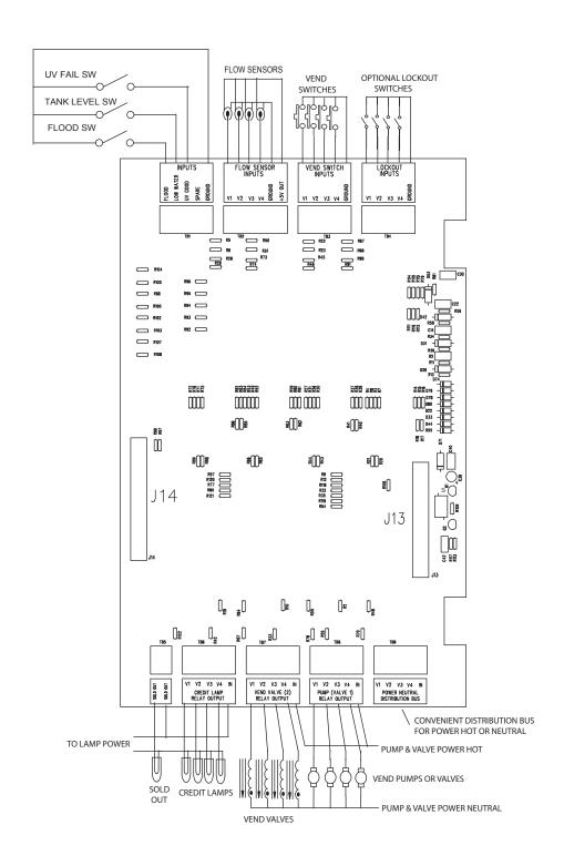
ESDI MODEL 110400 FOUR (4) STATION WATER VENDING MACHINE CONTROLLER WITH PAY STATION WIRING DIAGRAM
